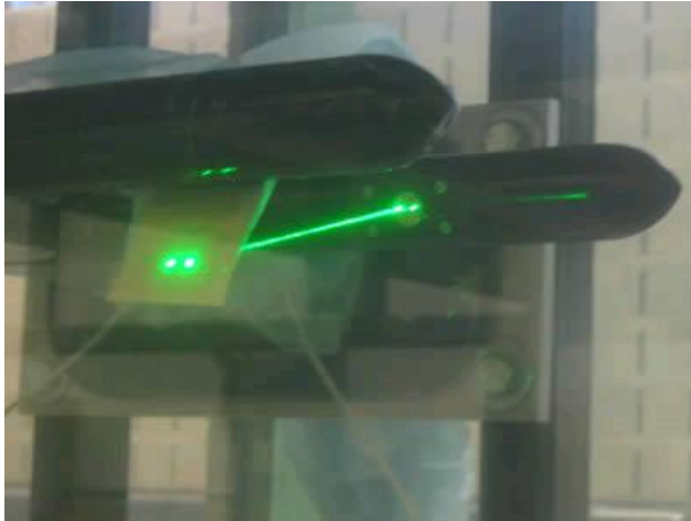
Figure 1: The Phase-Doppler Interferometer for Cloud Turbulence measuring droplets in the high-Reynolds-number, active grid wind tunnel at Cornell University.
