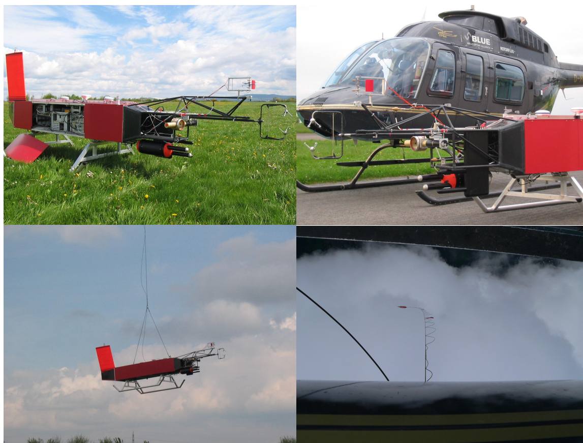
Figure 2: The ACTOS instrument payload (top left) and the helicopter used for deployment (top right). ACTOS during takeoff (bottom left), and a view from the helicopter looking down on ACTOS in the clouds (bottom right).
